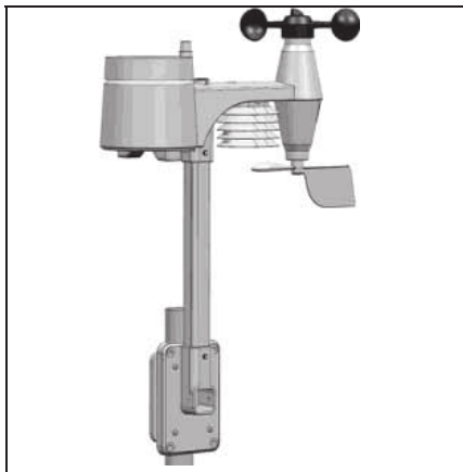
A. Mounting on pole (Pole Diameter 1"~1.3" (25~33mm))
